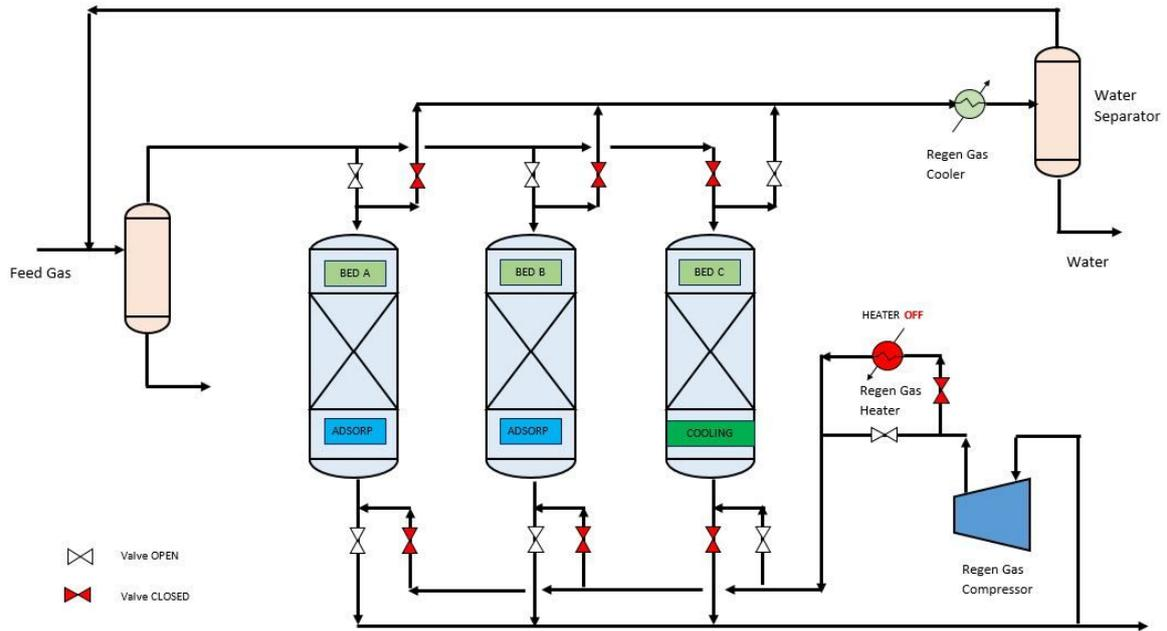
**Fig. A1:** Molecular sieve dehydration flow diagram – 2 towers in Adsorption and 1 tower in Cooling mode
