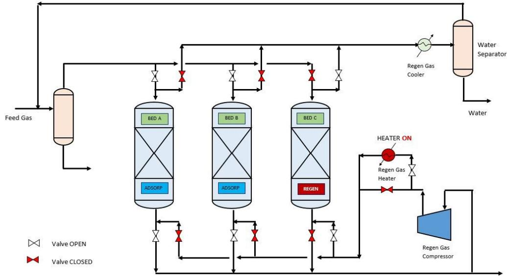
**Figure 3:** Molecular sieve dehydration flow diagram – 2 towers in Adsorption and 1 tower in Heating/regeneration mode
