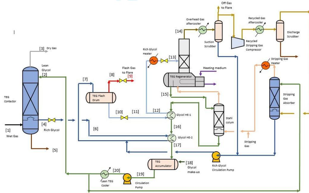
**Figure 4:** TEG dehydration unit with recycled stripping gas configuration
