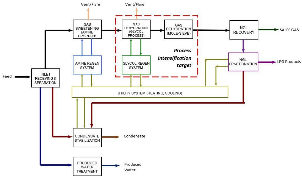
**Figure 1:** Typical block diagram in a natural gas plant in which gas was sweetened, and dehydrated before being processed in a cryogenic NGL recovery process
