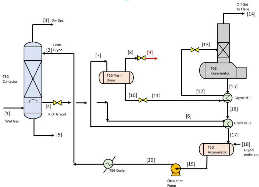
**Figure 2:** Conventional TEG dehydration unit for removing the bulk of water vapor
